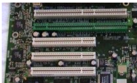
PCI slots 64 bit 5v 33Mhz and 3.3v 66Mhz (Example from Tyan Thunder motherboard)
